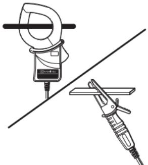
1. Clamp on the measured object and fix the Sensor. Firmly fix it so as not to easily come off.
