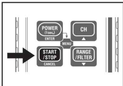
1. Press the **START /STOP** button at least 1 sec to stop recording.
