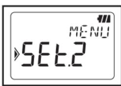
3. Press the **ENTER** button when "SEt.2" is displayed on the LCD.
