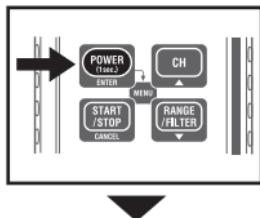
1. Pressing the
