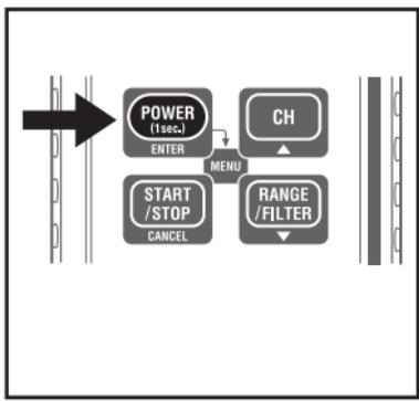
2. Press the **POWER (1sec.)** button at least 1 sec. to power on the instrument. Release the button when all indications are displayed on the LCD. First, time is displayed, and then sensors being connected are displayed. If incorrect time is displayed whenever powering on the instrument, internal battery for clock may be exhausted. In this case, send back the instrument to your local Kyoritsu distributor for repair.
