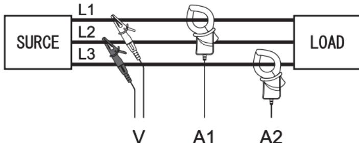
General formula is:  $P=V \times (A1 \times \cos(30^\circ - \Phi 1) + A2 \times \cos(30^\circ + \Phi 2))$ ,
