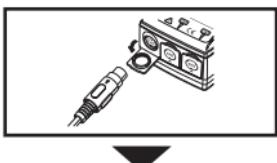
1. Connect a Sensor first prior to do setting.
