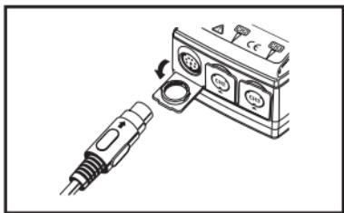
1. Press the **POWER (1sec.)** button and power off the instrument. Connect a Clamp/ Voltage Sensor to CH1 (for multiple connection, starting from CH1) while the instrument is being off. Connect them firmly with careful attention to the orientation of the connector.
