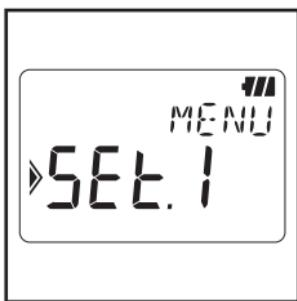
2. Press the **ENTER** button when "SEt.1" is displayed on the LCD.
