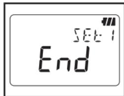
8. Now Setting 1 is completed; "End" is displayed on the LCD. Press the **ENTER** button to return to the screen on which "SET.1" is displayed.
