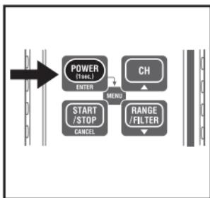
1. Power on the instrument, and press the **POWER** button. Then the instrument enters into Menu mode.
