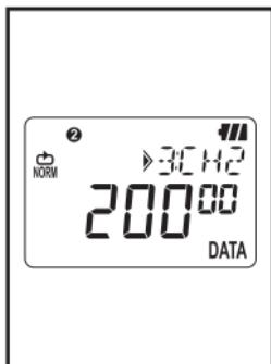
6. Display of the number of the recorded data at CH2/ the number of detected current & voltage data in case of Trigger Recording mode.
