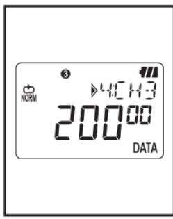
7. Display of the number of the recorded data at CH3/ the number of detected current & voltage data in case of Trigger Recording Mode.
