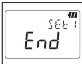
6. Now Setting 1 is complete; "End" is displayed on the LCD. Press the **ENTER** button to return to the screen on which "SET.1" is displayed.
