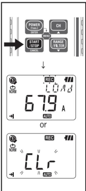
1. Press down the **START /STOP** button at least 4 sec. "**REC**" or "CLr" mark flashes. Keep the button pressed down until "**REC**" mark lights up. Recording stops when the button is released while the mark is flashing.
