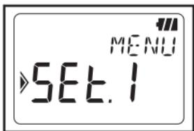
2. Press the **POWER** button while instrument is on to enter into Menu mode.
