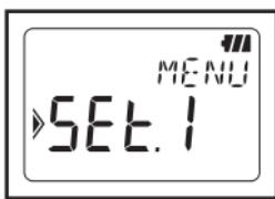
2. Press the **▼** button when "SEt.1" is displayed on the LCD.
