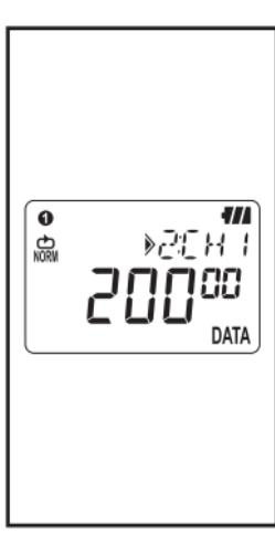
5. Display of the number of the recorded data at CH1/ the number of detected current & voltage data in case of Trigger Recording mode.
