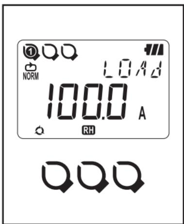
3. Check the connected Sensors. Sensor and the full-scale value are displayed.
