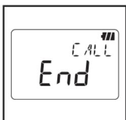
9. That's all for CALL Function to call the recorded data. Pressing the Button returns to the window with "CALL" message; pressing the Button closes Menu mode and gets ready for measurement.
